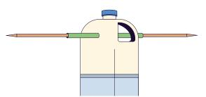
4. Insert the skewer into the straw. This is the base of the turbine ready to have blades mounted.
