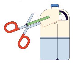
3. Push the straw through both of the small holes you cut into the bottle. Trim the ends of the straw so just a centimeter or two sticks out of each side.
